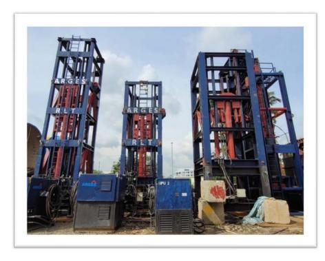
ARGES load testing systems are available with range from 14 Ton to 200 Tons. Our impact systems are designed to activate large range of test loads. The system includes guide frame, verticality adjustment hydraulic system, self-lifting hydraulic system and hold & release mechanism.
